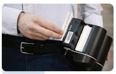
A wearable RFID tag encoder enables K-C workers or employees at a third-party packaging company to quickly encode the right EPCs for a specific batch of promotional displays.
