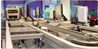
Hewlett-Packard Brazil created an RFID lab in Sao Paolo to test RFID equipment in the environment in which it would be used. The rollout was methodical and incremental. Since the RFID system went into full production in 2006, more than 2 million items have been tagged.
