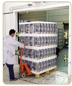
After the assembly is completed, the printers are moved to inventory transition points, or portals, at the manufacturing facility. Interrogators at the three portals track the printers as they are moved in and out of temporary storage areas.
